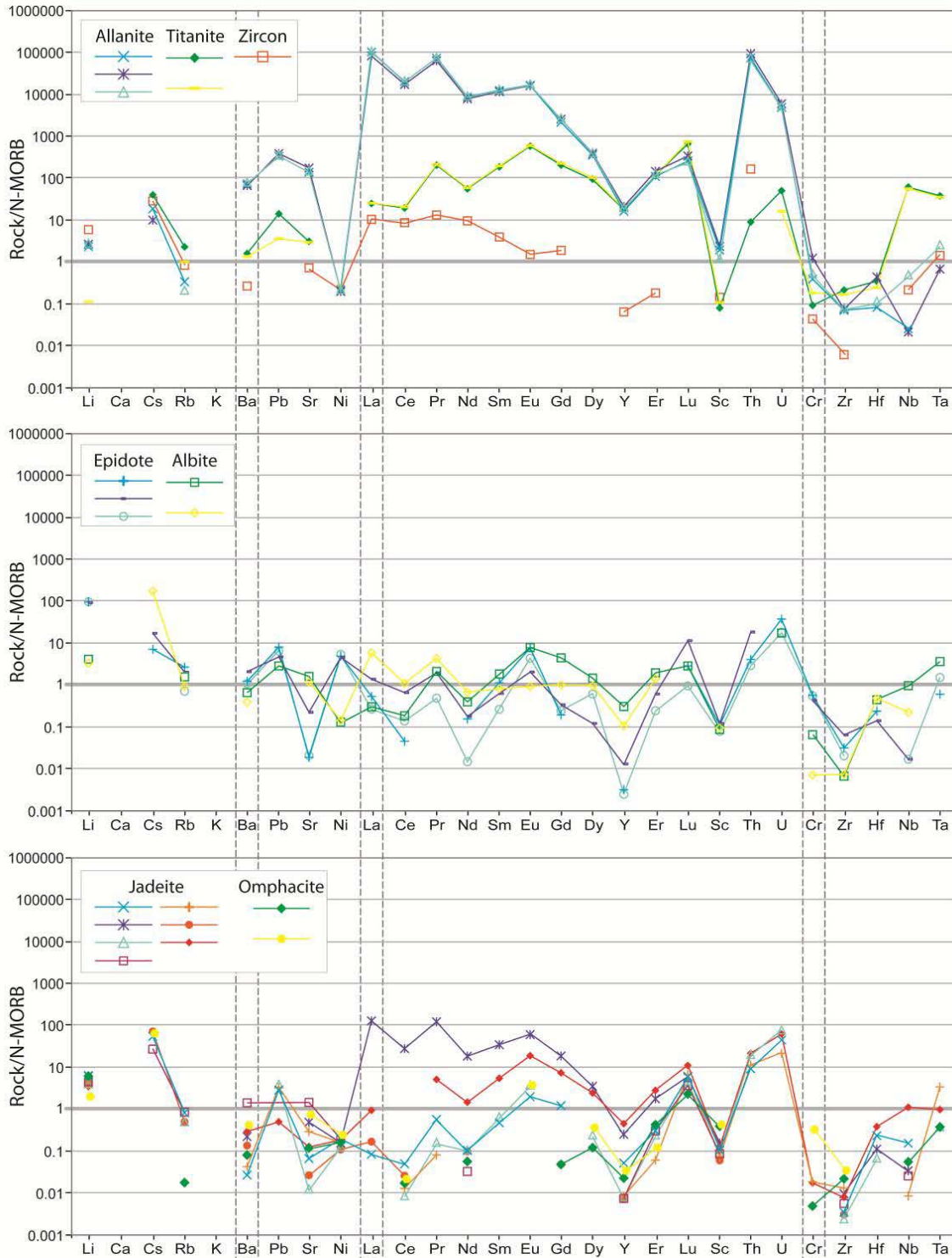
Figure 6.26. Trace element spidergrams for in situ LA-ICP-MS analyses of allanite, titanite, zircon, epidote, albite, jadeite and omphacite from pure jadeitite sample MCB-3h normalized to N-MORB (Sun and McDonough, 1989). Dashed rectangles indicate the key element used for ternary diagram of Cr-Ba-La ( \times 10 ).
