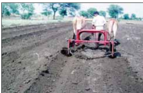
Fig. 8. A bullock-drawn Tropicultor bearing a fertilizer-cum-seed drill.
