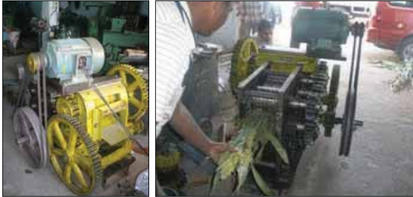
Fig. 7. The 3-pass 6-roller crusher and its testing.
