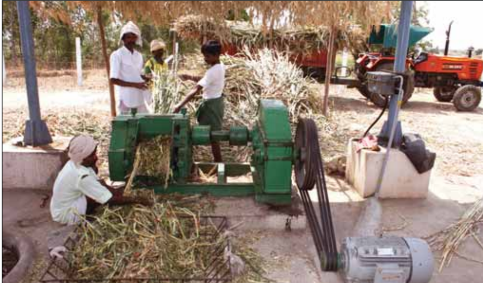
Fig. 2. Extraction of juice from sweet sorghum stalks.
