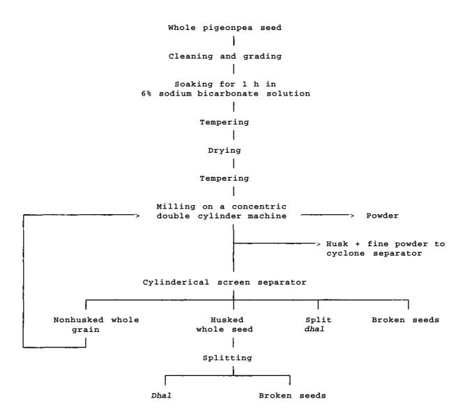
Figure 2.Flow chart of the improved Pantnagar dhal milling process.
