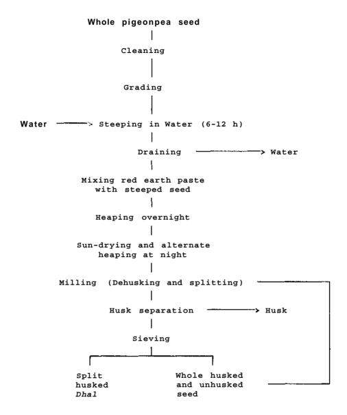
Figure 1. Flow chart for traditional milling of pigeonpea by wet method.
