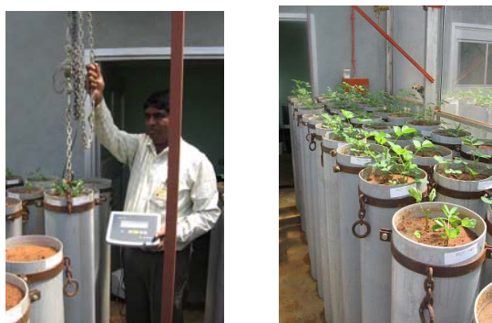
Figure 5. Use of PVC cylinders for root studies.
