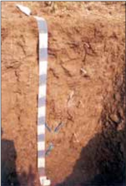
Closer view of the profile showing deep and wide cracks with well developed slickensides
