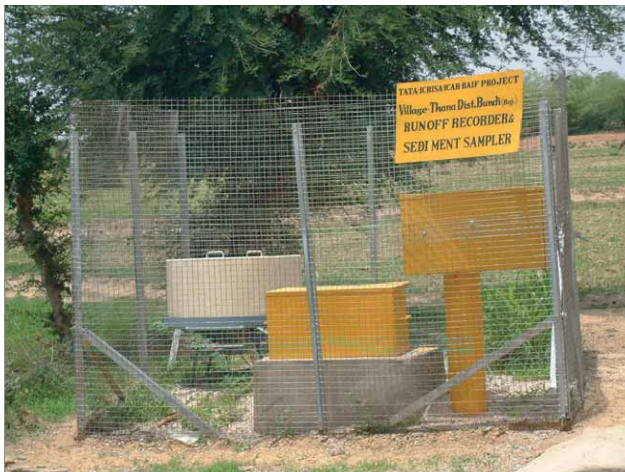
Figure 5. Hydrological gauging station for monitoring runoff and soil loss at Goverdhanpura watershed, Bundi, Rajasthan.
