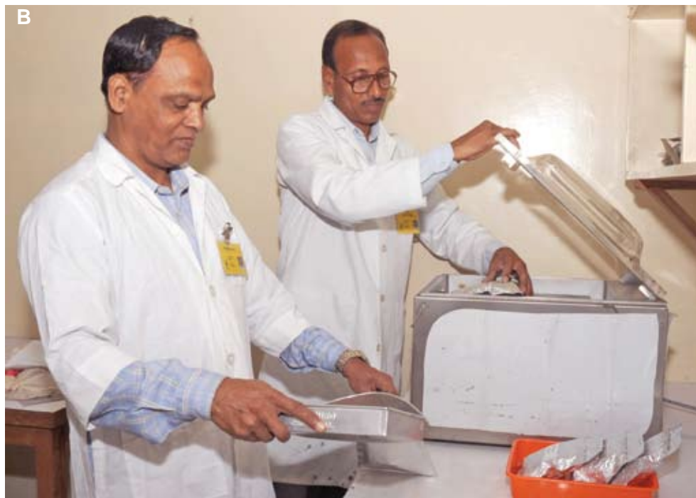
Figure 4F.2.1. Vacuum sealer (A) and packing seeds (B) for long-term conservation at ICRISAT genebank.
