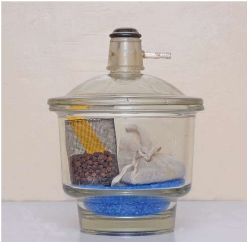
Figure 4C.2.1. Seed drying using silica gel at ICRISAT genebank.
