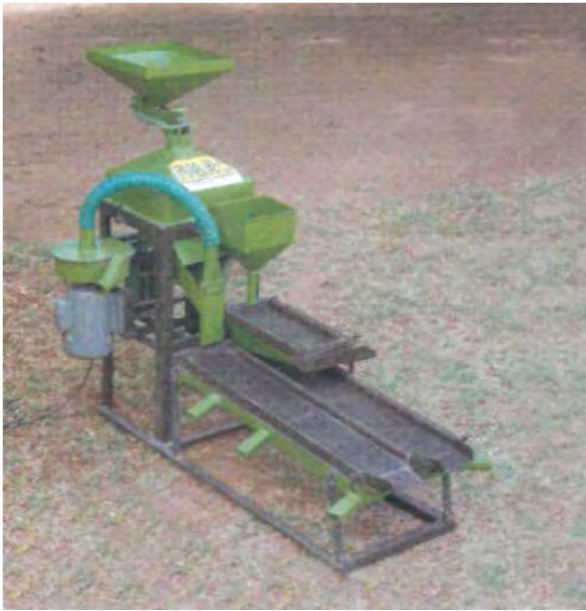
A small-scale pulse dehuller developed in Sri Lanka with support from the Asian Development Bank.
