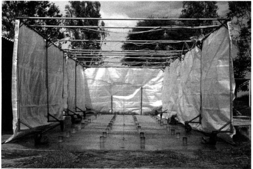
Figure 6 — Rainulator for studying infiltration under simulated rainfall conditions.
