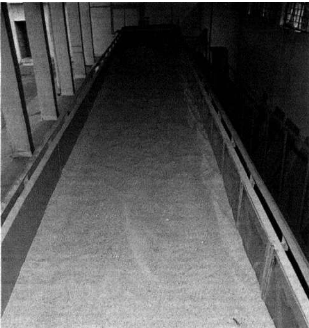
Figure 18 — A tilting flume assembly showing the tilting flume containing soil.
