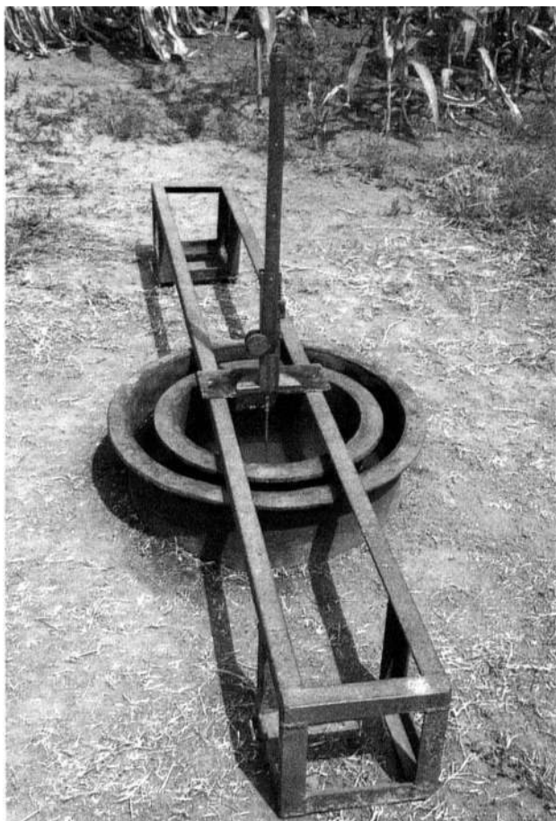
Figure 1 — Double-ring infiltrometer for measuring infiltration capacity of soil.
