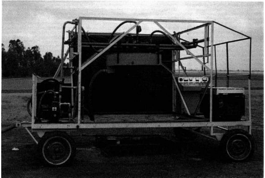
Figure 5 — Rainfall simulator for studying infiltration under simulated rainfall conditions.
