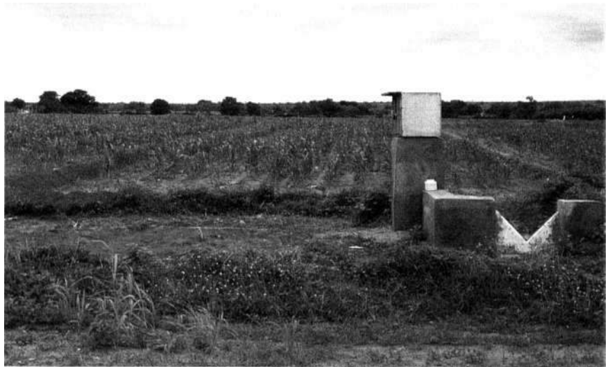
Figure 5 — A V-notch attached to a stilling well and connected to a drum-type recorder for measuring runoff.
