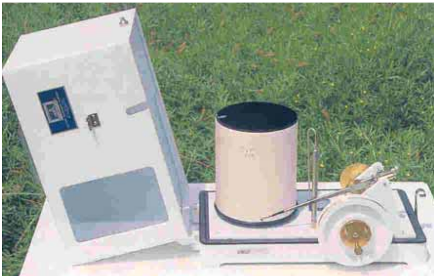
Figure 8. A drum-type mechanical runoff recorder.
