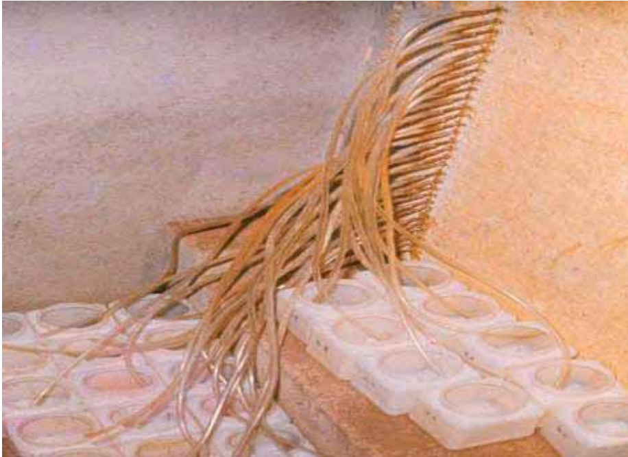
Figure 3. Depth integrating sediment sampler for small agricultural watersheds
