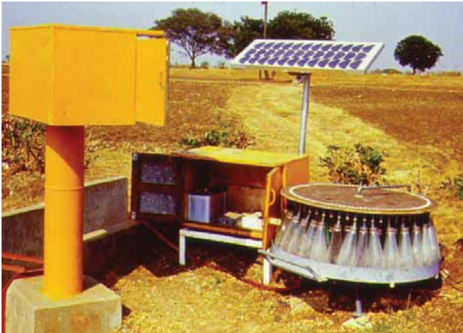
Figure 6. Microprocessor based automatic sediment sampler.
