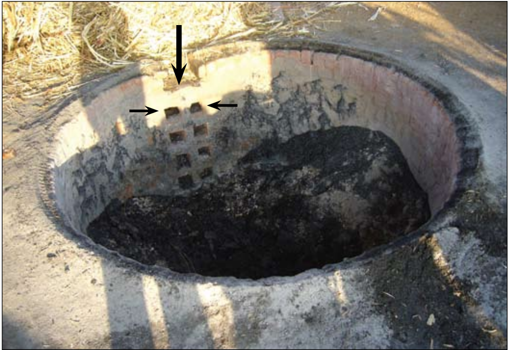
Figure 6. A chulha with its bagasse feeding opening (long arrow) and air passage channel holes inside the (short arrows) chulha.
