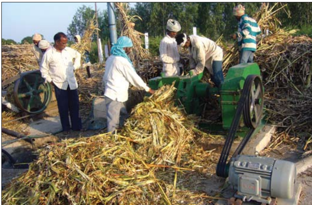
Fig. 10. Crushing of sweet sorghum stalk.
