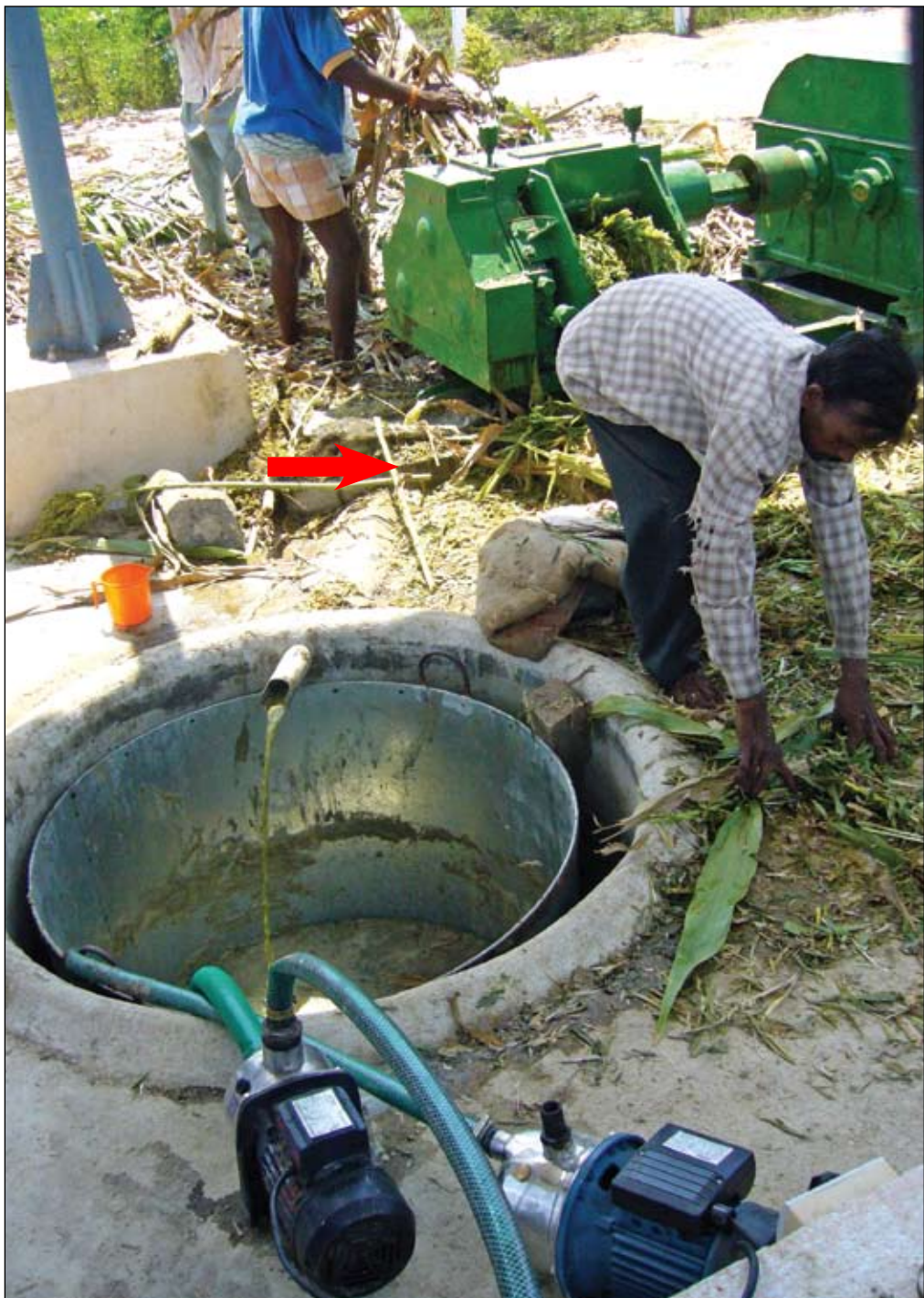
Figure 4. The juice collected in the drum is pumped in the syrup making pan using an electric motor.
