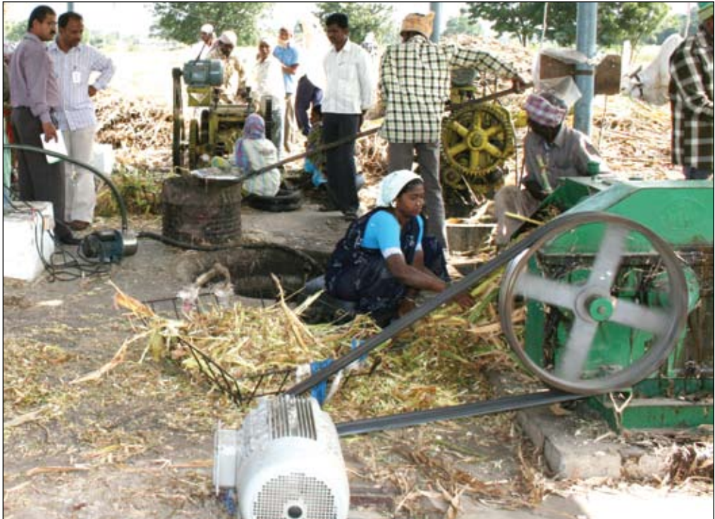
Figure 3. Crushing operations in progress where the motor is connected to the crusher with a pulley and V-belts.
