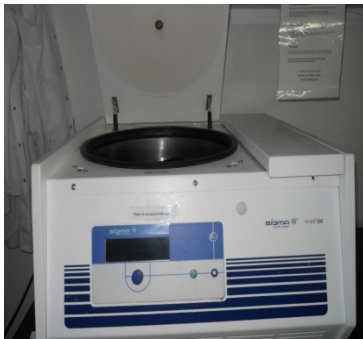
Centrifuge for ↓ spin upto 6000rpm
