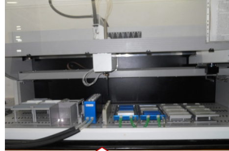
Robot machine ↑ used for dilution
