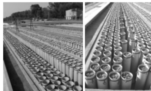
Fig. 7. Overall view of the lysimetric system developed at ICRISAT. The tubes are 1.2 m long with 20 cm diameter. They are filled with Alfisol at a set bulk density of 1.4. Each trench can accommodate approximately 700 cylinders. It takes about one day to 4 persons for weighing about 600 cylinders.
