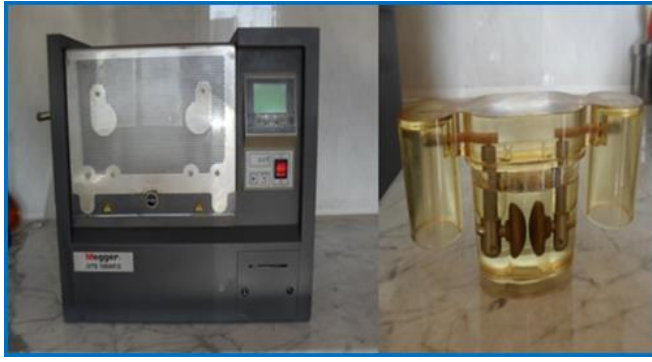
Fig.1. Megger OTS 100 AF/2 installation for breakdown testing the mineral: (a) general view, (b) testing oil tank.
