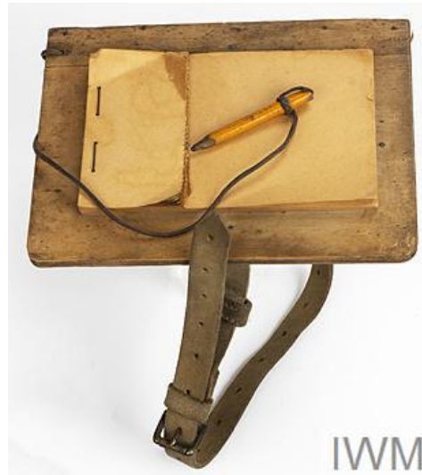
Figure 13: Knee desk, strapped to aviator's upper leg to enable him to make notes without disturbing his ability to operate his controls while flying (© IWM (EQU 3834)).
