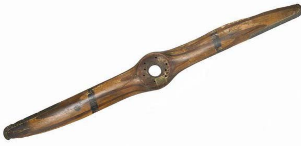
Figure 70: Wooden two-bladed propeller from a German Gotha GV aeroplane. Height: 204mm. Length: 310cm. Width: 356mm (© IWM (AIR 209)).
