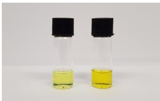
Figure A5.18. Compound 5.4 in the unimeric (chloroform, left) and aggregated (MCH, right) states.
