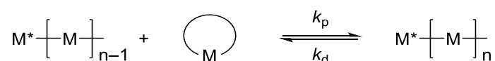
Scheme 1.1. The ROP of cyclic monomers, where k_p and k_d are the rate constant of propagation/depolymerisation, respectively, and M^* is the active species.
