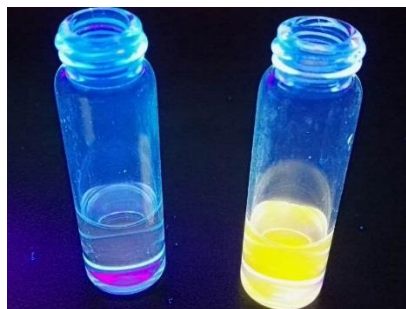
Figure 6.2. Photograph of 6.8 in MCH (0.02 mg mL -1 ), left: under air, right: immediately after N 2 was bubbled through the solution for ~15 sec.
