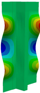
(d) Stringer buckling: 23.5 kN (Shell FE, left) and 24.5 kN (UF-SLE, right)
