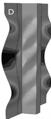
(e) Before collapse: 41 kN (Experiment, left), 39 kN (Shell FE, centre) and 39.5 kN (UF-SLE, right)
