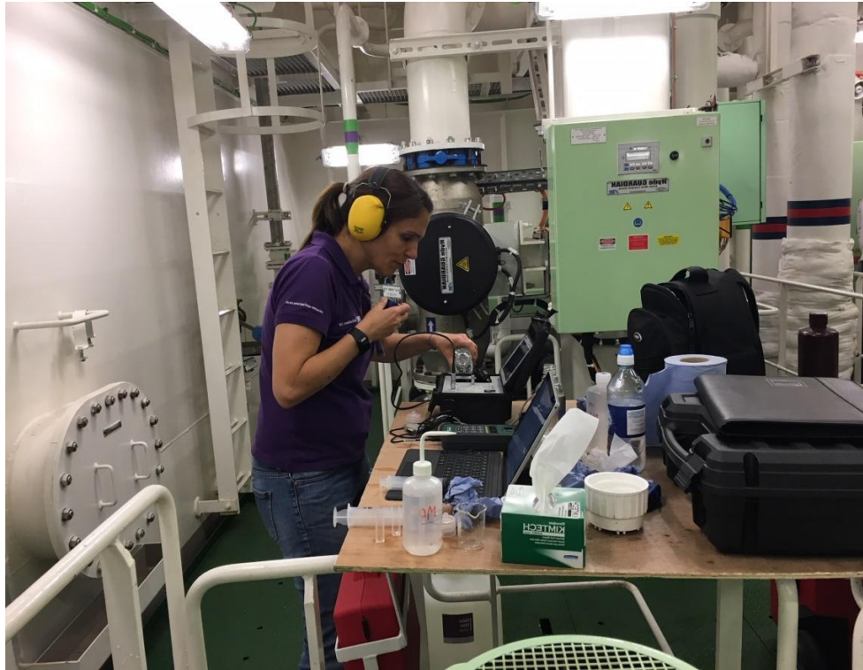
Figure 7.1. Testing treated ballast water samples with two portable fluorometers (Ballast Check 2 and FastBallast) during a ballast water shipboard efficacy test in Southampton, UK.
