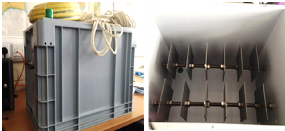
Figure 6.2. The simulated sea-chest built for the experiment (external and internal views).
