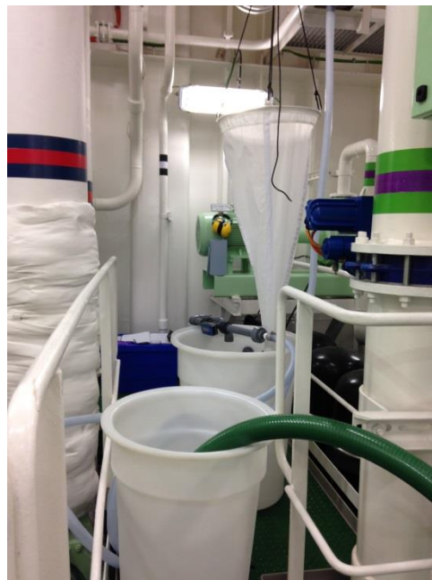
Figure 4.2. Sampling arrangements during ballast water shipboard tests.
