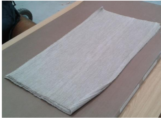
Figure 7.3: Flax-ply woven and UD fabric
