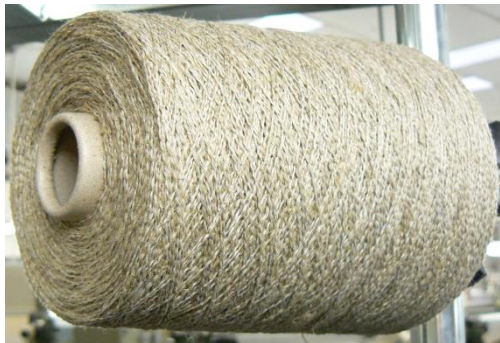
Figure 3.3: Flax fibre yarn roll produced by spinning technique (Courtesy of Composite Evolution)
