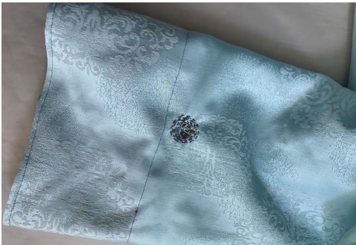
Figure 21: Detail of final version of dress sleeve and embroidered conductive thread button.
