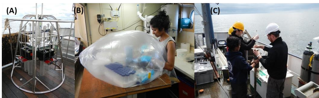
Figure 2.2. The Irish Sea mud-patch sampling campaign: (A) hydraulic mega-corer used to collect sediment cores from the mud-patch; (B) sampling of core in an \text{O}_2 -free atmosbag; (C) aerobic sampling of cores on deck.
