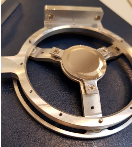
Fig. 3. Photograph of a degrader foil stretched over a degrader cone.
