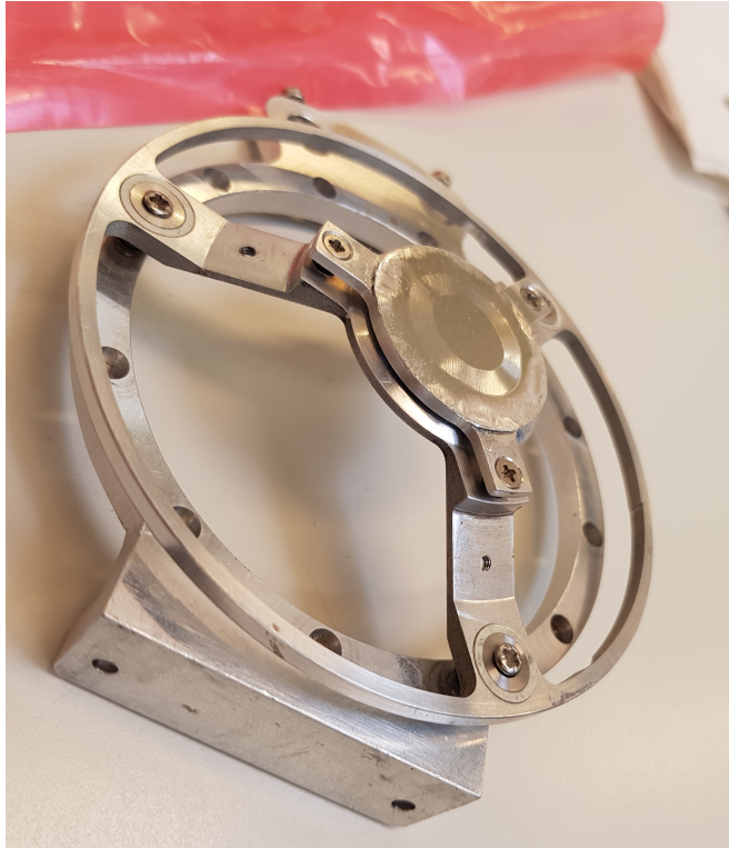
FIGURE 3.7: A photograph of a fully assembled foil frame and stretching cone ready to be screwed into the fixed target position. The cone is attached to the frame using the spring-screw mechanism described in Section 3.2.
