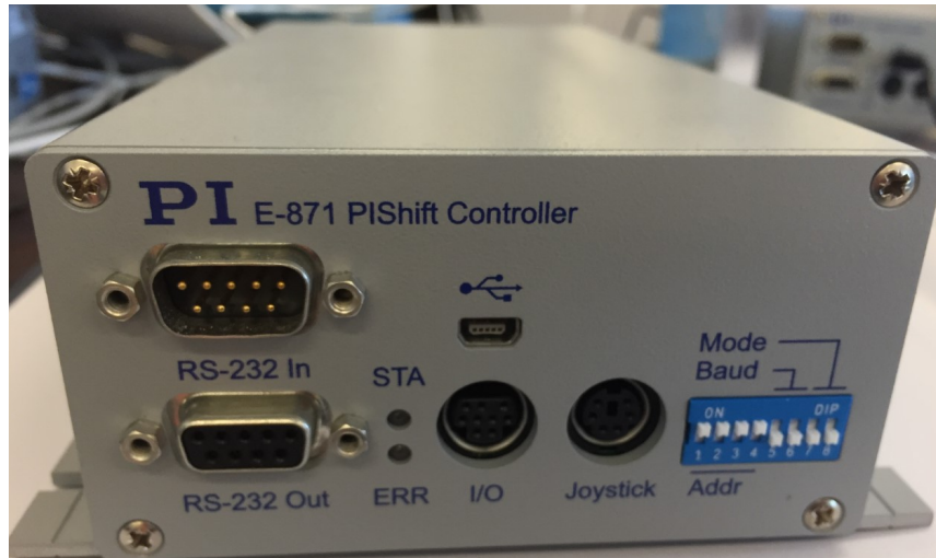
FIGURE 3.14: Photograph of the E-871 control unit used to control the motors. USB, RS-232 and joystick connections can be seen on the front face. Baud rate control and address switches are seen on the right hand side of the front face.
