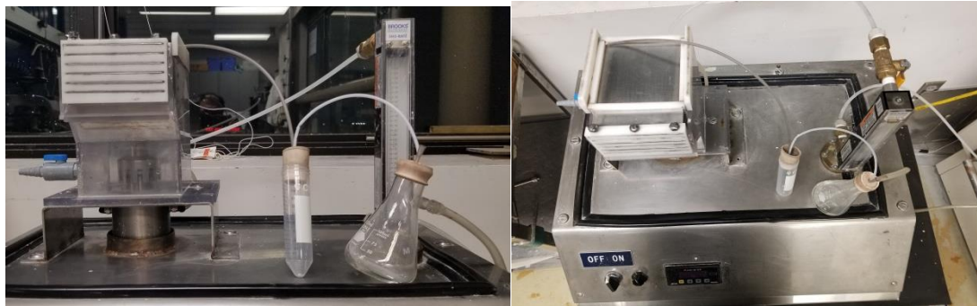
Figure 3.16: Vacuum apparatus to collect froth samples into a 50ml centrifuge tube (a) side view showing a conical flask used to catch any excess slurry. (b) top view showing the assembly
