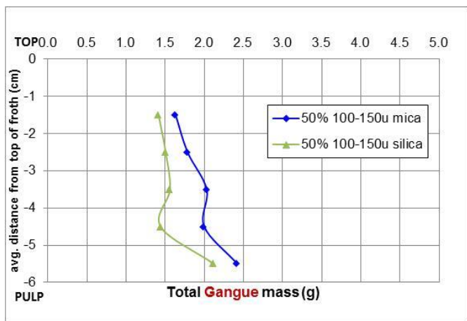
Figure 5.4: Nascent Froth sampling tests- Addition of 50% mica or silica of 20-50 \mu (a), 50-75 \mu (b), 75-100 \mu (c), 100-150 \mu (d) sizes to 50% fine silica. The plot shows total gangue mass (including mica and silica) in each layer. Solids concentration in pulp is 35%, and no chalcopyrite (sulfide value) is added. The total mass of gangue is significantly higher for 75-100 \mu and 100-150 \mu mica mixtures as compared to silica mixtures of the same size.
