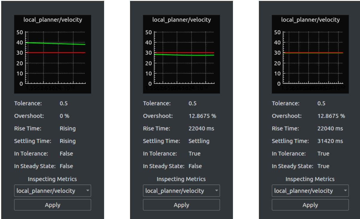
Figure 11: An example of the steady state analysis widget in the ground station. The velocity controller response starts from 50 m/s, shown in green, with a target step input of 30 m/s, shown in red. The three pictures, from left to right, show the determination of overshoot, rise time, and settling time metrics of the controller response.
