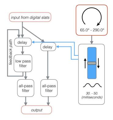
Figure 6.14: A diagram of the modulation of the cloth pitch.
