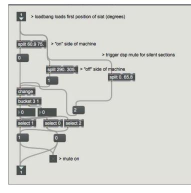
Figure B.11: Activating and Muting the Digital Slat in Max/MSP.
