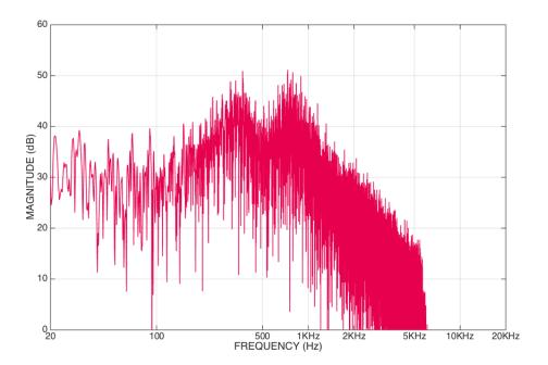
Figure C.12: Spectrogram of the second iteration of the prototype digital wind machine.
