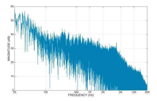
Figure C.2: Spectrum of the acoustic wind machine.
