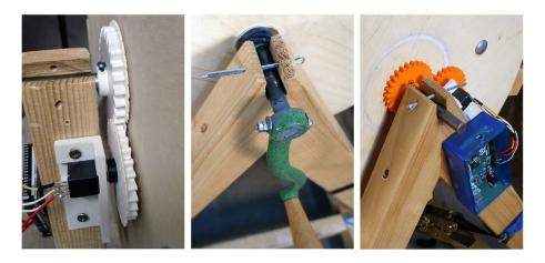
Figure 6.3: (L-R) Fitting the first gearing prototype with the rotary encoder's spacer, adding a spacer between the cylinder and axle, and the final configuration of laser cut gearing, rotary encoder and Arduino on the acoustic wind machine, with grind marks evident on the plywood.
