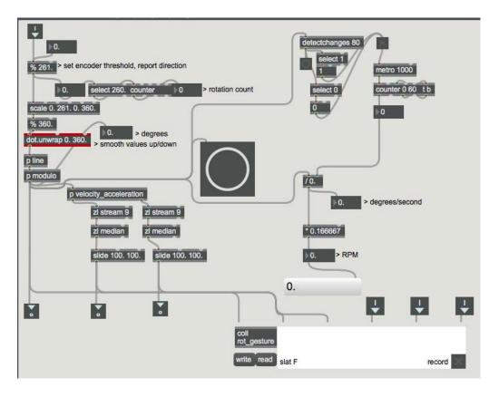
Figure B.6: Rotational Smoothing and Data Recording in Max/MSP.
