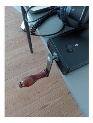
Figure 6.25: The second iteration of the digital crank interface.
