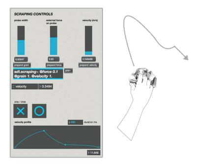
Figure 6.10: (L) The controls to [sdt.scraping~] as offered by its Max/MSP help file. The velocity profile on the bottom automatically triggers the scrape by moving the velocity slider up steadily, and then down more slowly. (R) How that velocity profile might perceivably suggest the shape of a real-world scraping action with a crumpled ball of paper to a listener.
