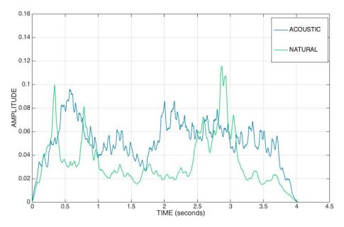
Figure 5.15: A comparison of the amplitude envelopes of a particularly frenetic and high-pitched whistling natural wind sound (green) and the acoustic wind machine (blue) imitating that sound.
