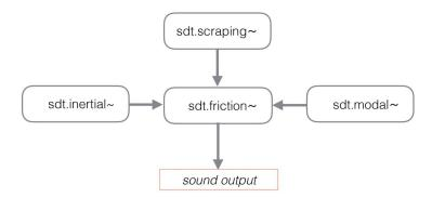
Figure 6.8: The configuration of SDT objects used to model the sound produced by each of the acoustic wind machine's slats in interaction with the cloth.
