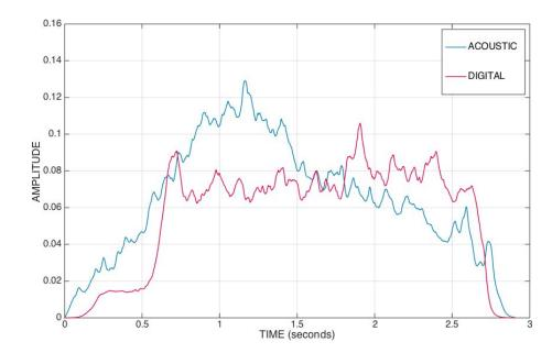
Figure 6.16: A comparison of amplitude envelopes for the same single rotation of the acoustic wind machine and the prototype digital wind machine programmed in Max/MSP.
