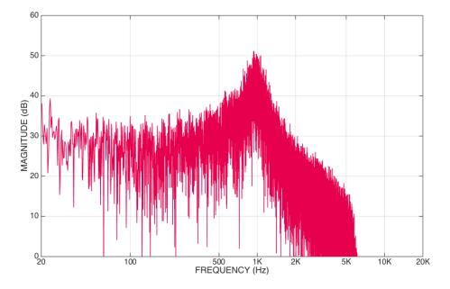
Figure 6.20: Spectrum of Digital Wind Machine (1 rotation)
