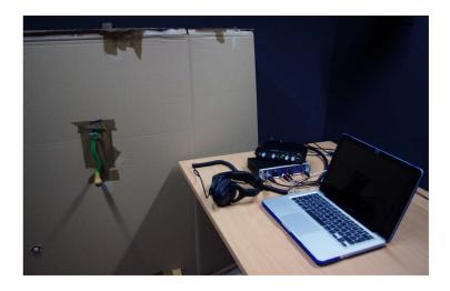
Figure 4.7: Concealing the acoustic wind machine to remove any visual feedback for the experiment.
