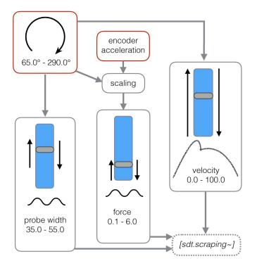
Figure 6.13: The real-time modulation of the probe width and force sliders for each  $[sdt.scraping\sim]$ .
