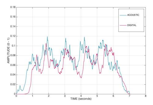
Figure C.14: Comparison of the amplitude envelopes for 5 rotations.
