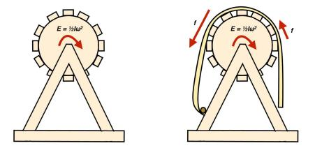
Figure 5.14: (L-R) The acoustic wind machine without its cloth, free to accumulate rotational energy, and the direction of the frictional force exerted by the cloth on the cylinder's motion which shape the performance gesture into two perceivable parts.
