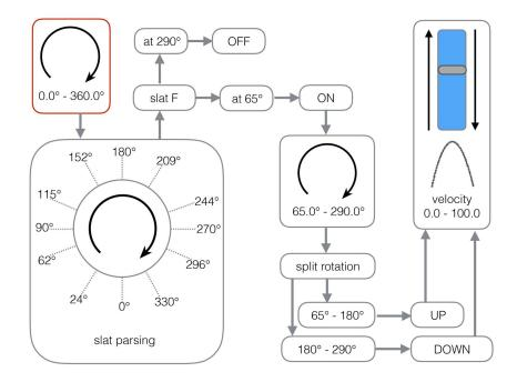
Figure 6.11: The main rotational data from the rotary encoder is parsed to create twelve individual streams, which are then tracked to facilitate DSP muting. The rotational movement of each digital slat is also converted to a linear movement to move the velocity slider up and down, producing sound from [*sdt.scraping*~].
