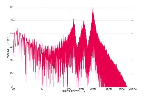
Figure C.7: Spectrogram of the first iteration of the prototype digital wind machine.
