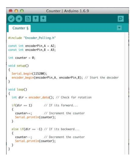
Figure B.1: Rotary encoder program in the Arduino IDE.
