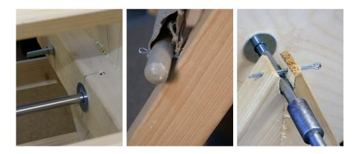
Figure 5.8: Split pins used to (L-R) fix the steel rod axle to the cylinder, fix the cloth to the frame, and fix the rotating axle onto the frame.
