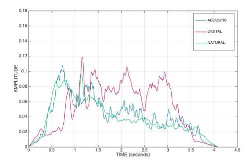
Figure 7.2: A comparison of amplitude envelopes for the gusty Acoustic (blue), Digital (red) and Natural (green) wind sounds.
