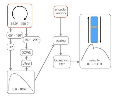
Figure 6.12: Adding complexity to the velocity slider data for each digital slat, with the addition of an offset, scaling according to the main rotational velocity of the encoder, and a logarithmic filter.
