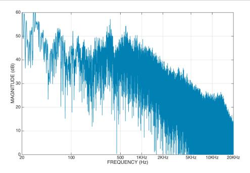
Figure C.6: Spectrogram of the acoustic wind machine.
