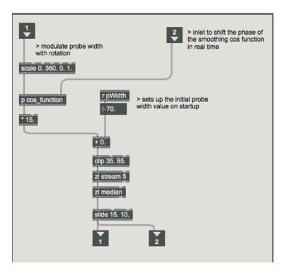
Figure B.13: Real-Time Modulation of Probe Width Parameter in Max/MSP.
