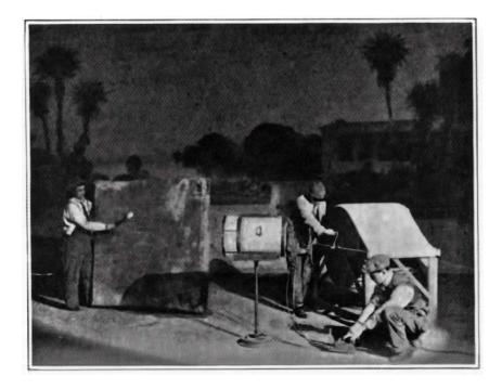
Figure 3.2: Some of the theatre sound effects apparatus from Century Theatre. A square thunder drum can be seen on the left, and a wind machine on the right. The original caption reads "Thunder drum for rain and reverberating thunder, lightning flasher and wind machine" (Scientific American, 1913, p.378). Image included here courtesy of Scientific American.
