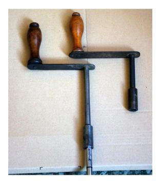
Figure 5.5: Fitting a Victorian table winder handle to the steel rod axle.
