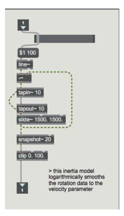
Figure B.8: The Logarithmic Filter/Signal Inertia Model in Max/MSP.
