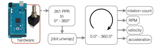
Figure 6.5: Diagram of the first part of the Max/MSP program, which captures the acoustic wind machine's movement as rotational data, smoothing it to a range of  $0.0^{\circ}$ -360.0°, and then calculates some additional data from this continuous rotation.
