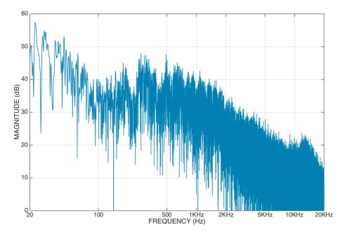
Figure C.11: Spectrogram of the acoustic wind machine.
