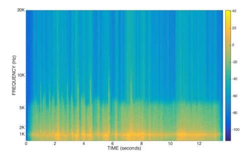
Figure 6.22: Spectrogram of 10 rotations with the prototype digital wind machine.
