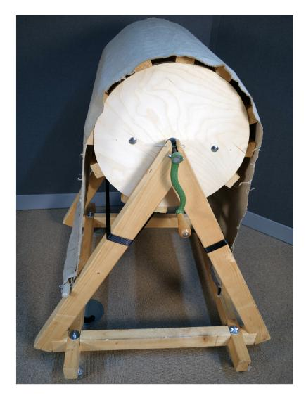
Figure 5.11: The completed acoustic wind machine with ratchet strap and wheels.
