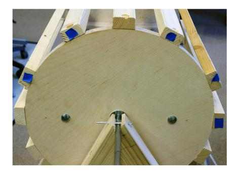
Figure 5.7: The final placement of the slats on the acoustic wind machine.
