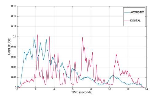
Figure 6.18: A comparison of amplitude envelopes for the same ten rotations (starting at speed and then diminishing in energy) of the acoustic wind machine and the prototype digital wind machine in Max/MSP.
