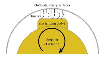
Figure 6.7: Diagram of the bristle interpretation of friction used within the SDT model and how it might be applied to the interaction between each wooden slat and the rough cloth (based on Fontana & Rocchesso (2003, p.152))
