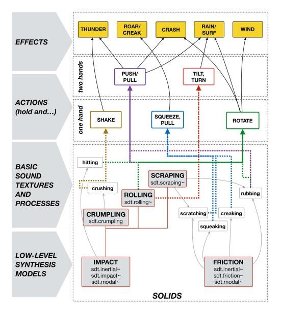
Figure 3.13: Expanding the Sound Design Toolkit (SDT) (Baldan et al. 2017) with the action-sound configurations of theatre's acoustemology in the late nineteenth and early twentieth century.
