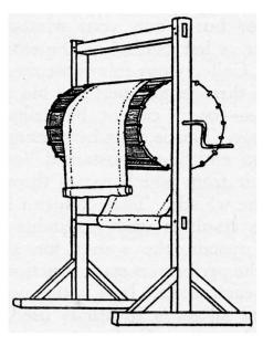
Figure 5.4: Wind machine design by Napier from his "Noises Off" (1962, p.51). Image used here with permission of Cressrelles Publishing Co. Ltd.
