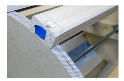
Figure 5.9: A slat after chamfering and sanding. The countersunk screw can also be seen fixing the slat to the plywood disc.
