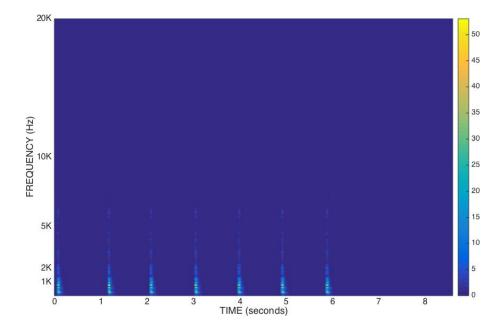
Figure 4.5: A spectrogram of the same sound of a hammer hitting a nail, produced with MIR Toolbox in MATLAB.
