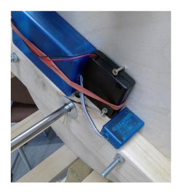
Figure 6.2: The initial configuration of (L-R) an Arduino and transmitter, battery pack and IMU sensor installed on the acoustic wind machine.
