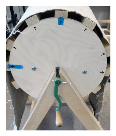
Figure 5.16: The acoustic wind machine at rest. The arrows mark each of the seven slats in contact with the cloth.
