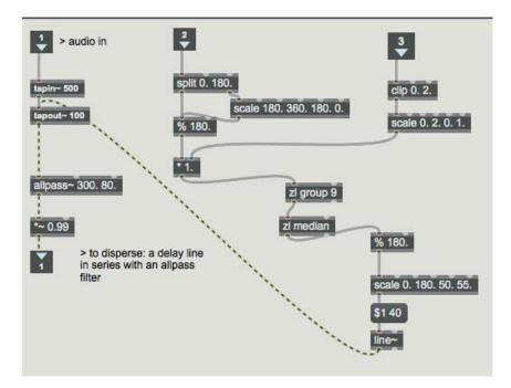
Figure B.14: Dispersion for Each Digital Slat in Max/MSP.
