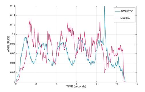
Figure 6.17: A comparison of amplitude envelopes for the same five rotations of the acoustic wind machine and the prototype digital wind machine programmed in Max/MSP.
