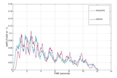
Figure C.15: Comparison of the amplitude envelopes for 10 rotations.
