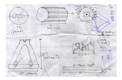
Figure 5.6: An extract of the cutting list produced for the acoustic wind machine, with layers of notes added during the construction process as the parts took shape.
