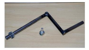
Figure 6.23: The first iteration of the digital crank handle and the digital rotary encoder it turned.
