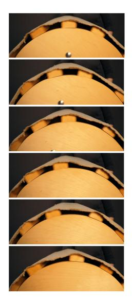
Figure 5.18: Video stills showing the shifting motion of the cloth against the wooden slats during rotation.
