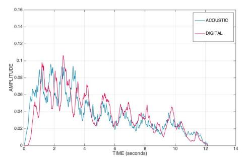
Figure 6.15: An amplitude envelope for 10 rotations starting at speed and diminishing in energy performed with both the acoustic wind machine (shown in blue), and an early iteration of the prototype digital wind machine (shown in red) before some responsive whistling behaviour was added to its program (First published in Keenan & Pauletto (2017a)).
