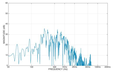
Figure 4.4: A spectral analysis of the sound of a hammer hitting a nail, produced with MIR Toolbox in MATLAB.
