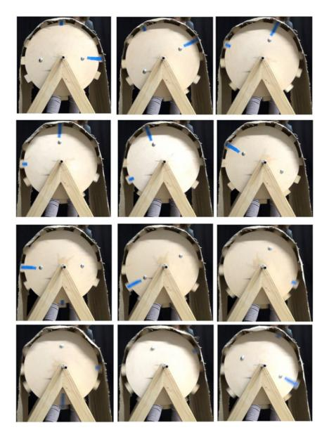
Figure 5.17: Video stills showing the slat movement through one rotation of the wind machine's handle. Rotation is anticlockwise when viewed from this side of the machine.
