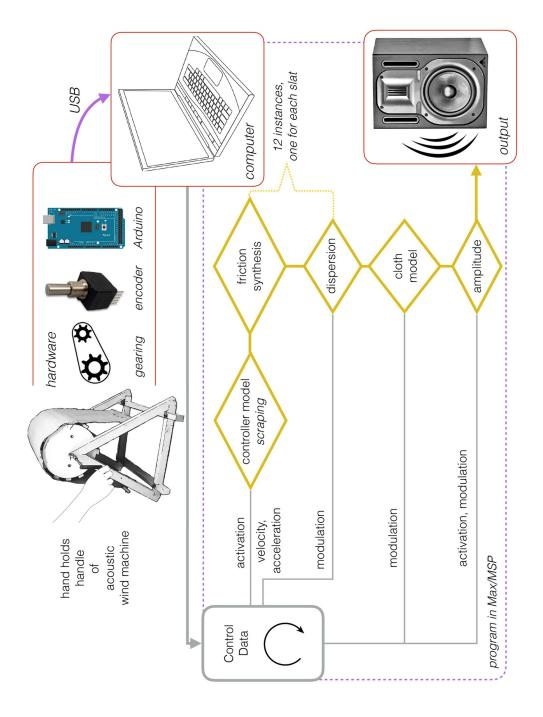
Figure 6.1: The main components of the prototype digital wind machine presented in this chapter.
