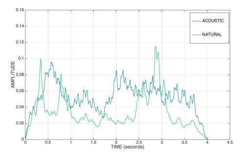
Figure C.1: Amplitude envelopes for the same gesture with the acoustic wind machine (blue) and the natural wind (green).
