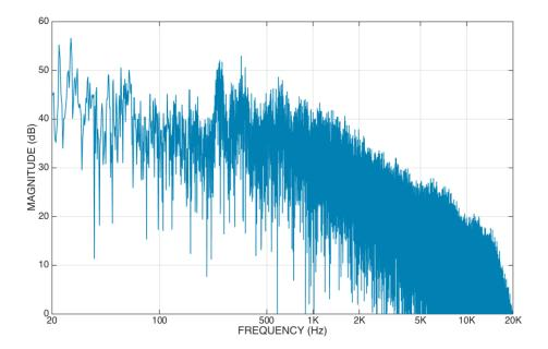
Figure 6.19: Spectrum of the Acoustic Wind Machine (1 rotation)
