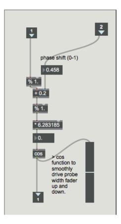
Figure B.12: Cos Function for Modulation in Max/MSP.
