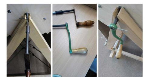
Figure 5.10: (L-R) The first iteration of the wind machine's crank handle showing the development of the twist in the axle, working to fabricate the new meat grinder handle and axle, and fitting the new crank handle and axle.
