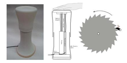
Figure 2.7: (L-R)The Spinotron, its internal mechanism and the virtual mechanism of its sound model. Images used here with permission of Karmen Franinović.
