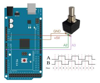
Figure 6.4: Wiring diagram showing the pin connections between the rotary encoder and Arduino prototyping board (left), and the encoder A/B input that it monitors to produce incremental degree values (right). The Arduino sends 5 volts of power to the encoder, and reads the A and B quadrature outputs as it turns.
