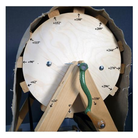
Figure 6.6: Side view of the acoustic wind machine with its slat positions marked in a 360° clockwise rotation from their position of origin. The degree values used to parse each slat position from the main data stream in Max/MSP and replicate those positions digitally are also shown.
