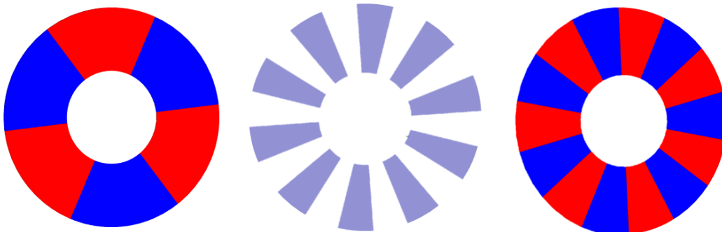
Figure 4. HSR with 3 pole pairs. 10 Modulator pieces. LSR with 7 pole pairs. (Left to Right)
