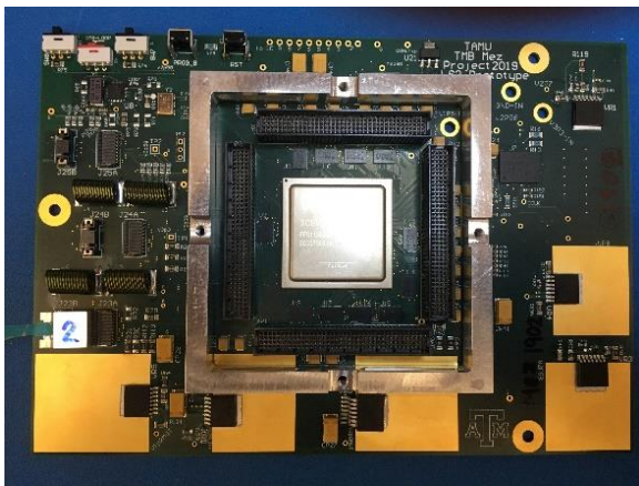
Figure 6. Circuit Board Used For Future SEU Testing of Optical Devices.
