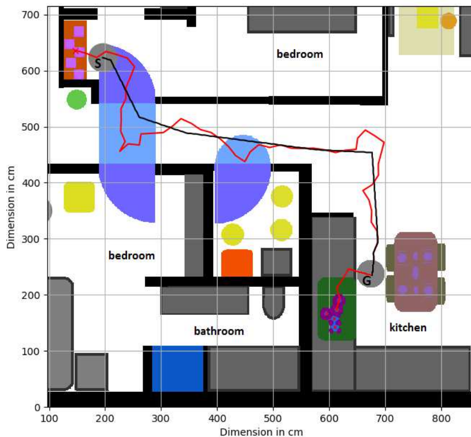
Fig. 2. Robot skill: move objects to a region. The robot moves all objects (purple dots) from the shelf (brown) in the bedroom to the sink (green) in the kitchen. The black line shows the smoothed robot path.
