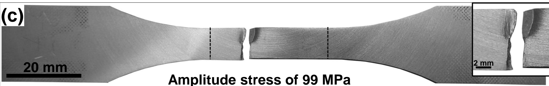
Figure 7. Typical appearance of specimens failed during fatigue tests: base material (a), the weld fatigued at relatively low stress and failed in the base material zone (b), and the weld fatigued at relatively high stress and failed in heat-affected zone (c). The magnified images of fracture surfaces are shown in the top right corners of the figures. The dotted lines show gauge area. See Section 3.4 for details. Note: The amplitude stresses are specified below the specimens.
