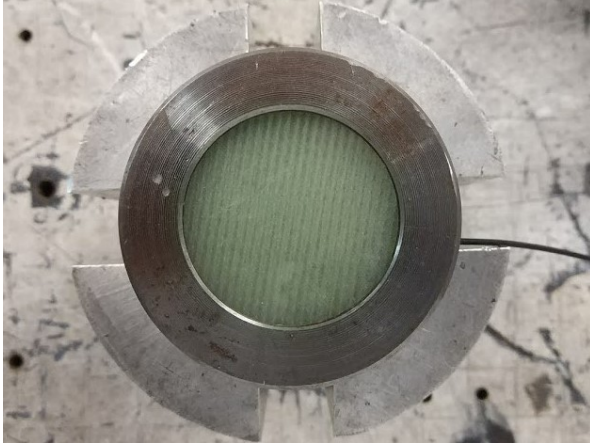
Figure 4: Composite clamping arrangement with force transducer attached.
