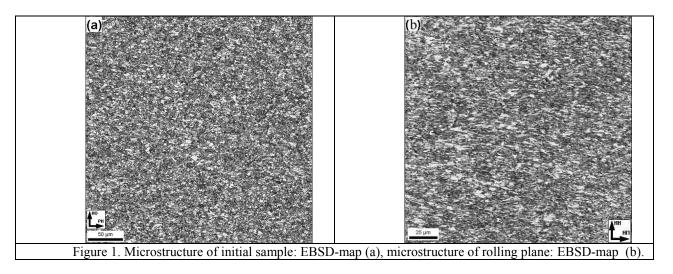
The analysis of the developed texture demonstrated that the plastic flow arises mainly from conventional {111}<110> slip. The cryogenic rolling was shown to increase strength and decrease ductility (Tab.) and both effects might be attributed to the substructure.
