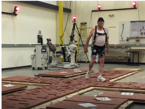
Fig. 1: Experimental setup for gait trial data collection showing an older adult participant performing a 90° online turn to the left. Interchangeable flat surface panels and strength testing equipment also shown.
