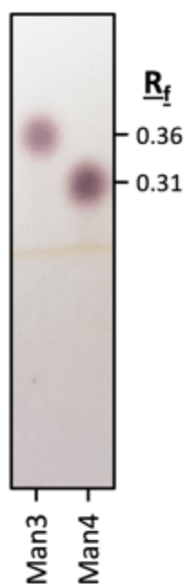
Appendices 6. 13 – TLC analysis of \beta -(1-2)-mannotriose and \beta -(1-2)-mannotetraose \beta -(1-2)-mannosides. Solvent system - BuOH/EtOH/H 2 O (10:8:7).
