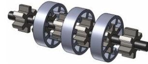
Fig.12. A multi-stator RL SR motor [30].
