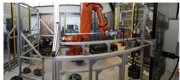
Fig. 6. Setup for identification of joint stiffness of a robot.
