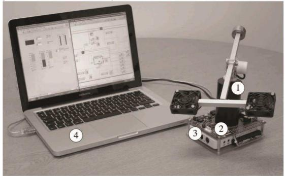
Figure 4: Example of a take home helicopter kit [1] which students can connect to their laptops via a USB
