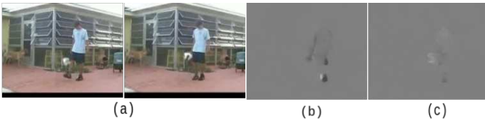
Fig. 1: (a) consecutive pair of images (b) and (c) horizontal and vertical component of optical flow
