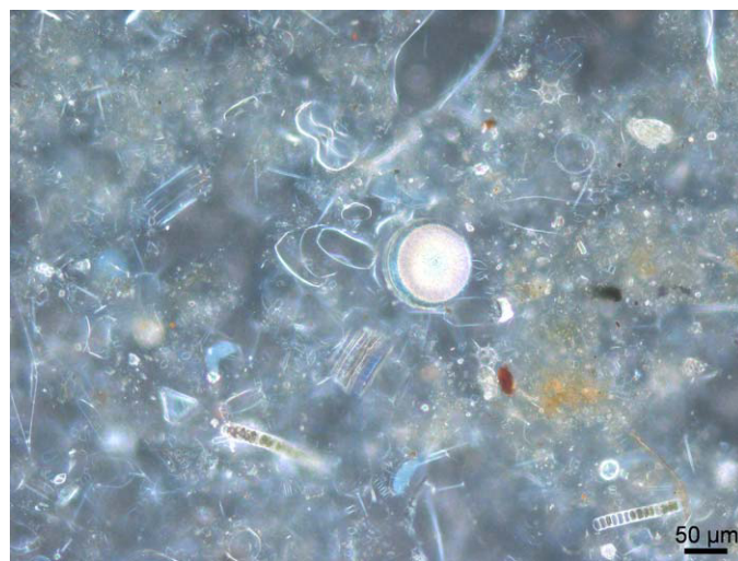
Fig. 3. Bright-field micrograph of an 80 \mu\text{m} thick slice through an Araldite 502 embedded aggregate formed from surface water off Helgoland, Germany. The resin did not allow structural staining, but valves and pigments are clearly visible. Araldite 502 sections are also amenable to NanoSIMS.
