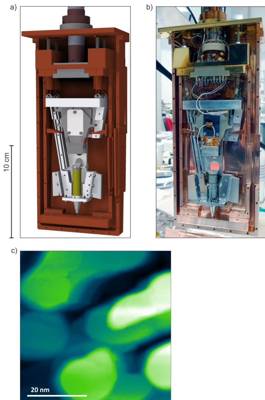
Figure 4.15 (a) 3D drawing of the final design of the THz-STM. (b) Picture of the assembled STM prior closing the shell and radiation shields. (c) Constant current topography recorded on a Gold on Mica surface showing terraces with atomic steps (junction setpoint 1 nA at 1 V).
