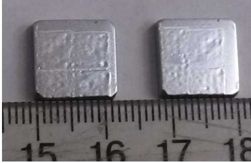
Fig. 1. Eurofer samples after damaging with e-beam in JUDITH-1. Pulse duration is \Delta t=1 ms, absorbed power density is 0.71 \text{ GW/m}^2 , and pulse number is 10.
