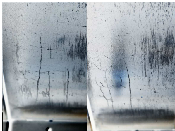
Figure 2. Foto of 2 strike point tiles of the massive W divertor III after 2 campaigns. Each tile has a width of 74 mm, a height of 213 mm and a thickness of 15 mm.
