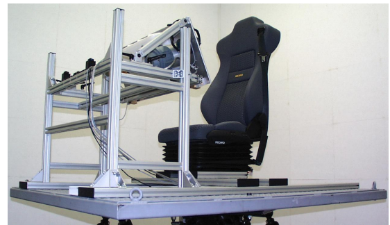
Figure 20: Driving setup with force feedback steering wheel.
