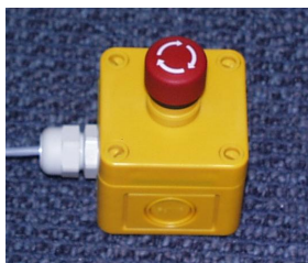
(c) emergency break for the subject on the platform
