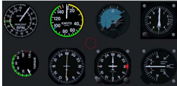
Figure 21: The layout of instrument panel of a Bo105 model from Flightgear; the red circle in the center of the panel represents the 1.5° resolution of the eyetracker (not shown during experiments).
