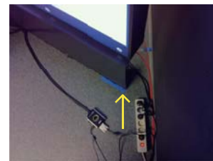
(c) A color line assists to position a monitor deck on the right side (pointed with a yellow arrow)
