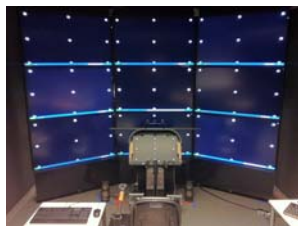
(a) A flight simulator (color lines on the floor are used to calculate coordinate information of each device)
