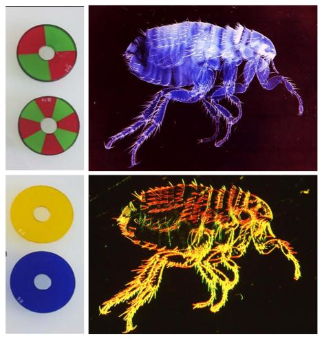
Figure 3. Microscopic image of a flea viewed with Rheinberg contrast in which arbitrary colors are generated by color filters in the aperture plane. Left: Selection of Rheinberg filters of which the peripheral ones define the specimen color and central filters the background color. Right: images obtained with a central black stop and a peripheral four zone filter similar to the one on top but with different colors. Photo Live Cell Imaging Center Rostock, courtesy of Willi Maile.
