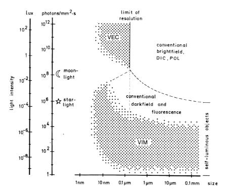
Figure 10. Video microscopy works beyond the limits of conventional light microscopy. When plotting light intensity against object size, the new application areas for video microscopy are seen (dotted areas) both in low light situations (VIM) and when working with very small objects (VEC microscopy). Modified from Weiss et al. 1998.
