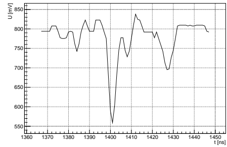
(a) Example signal of the recorded photo-current. (b) Parasitic signal some time after the signal in (a)
