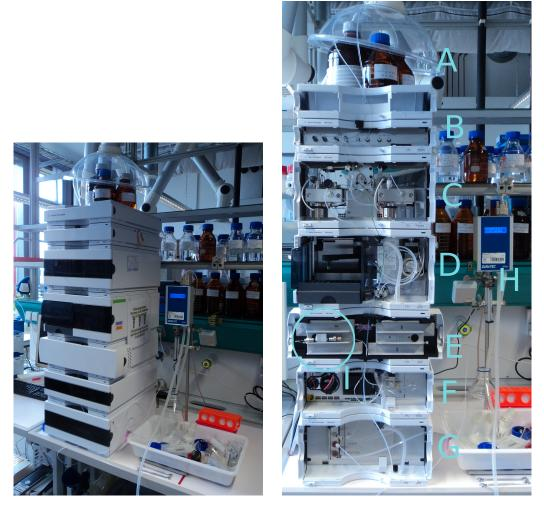
Figure A1: Agilent 1260 HPLC station used for experimental investigation of Part III. Components and part numbers: A: liquids & solvents; B: degasser (G1322A); C: dual pump module (G1312C); D: sampler & injection loop (G1329B); E: column compartment & oven (G1316A); F: multiple wavelength detector (G1365D); G: refractive index detector & waste outlet (G1362A); H: flowmeter; and Hypercarb<sup>TM</sup> column (I). Courtesy of *Physicochemical Fundamentals Group*, MPI Magdeburg.
