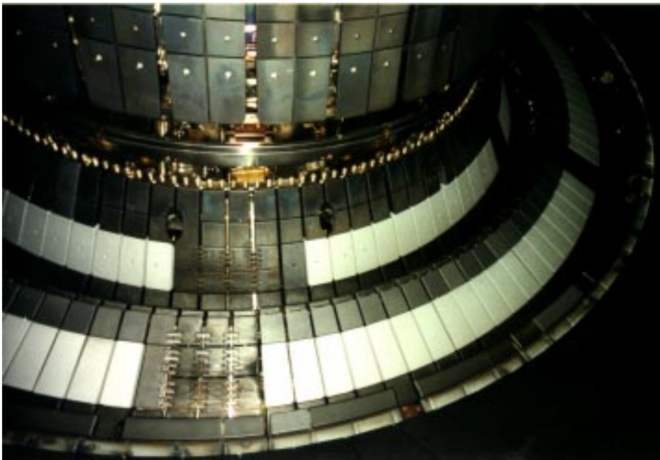
Figure 6.1: The tungsten divertor in ASDEX Upgrade. The tungsten coated tiles were mounted on a toroidal ring at the outer and the inner strike zones of Divertor I (DIV I). They are clearly visible as light grey rings.
