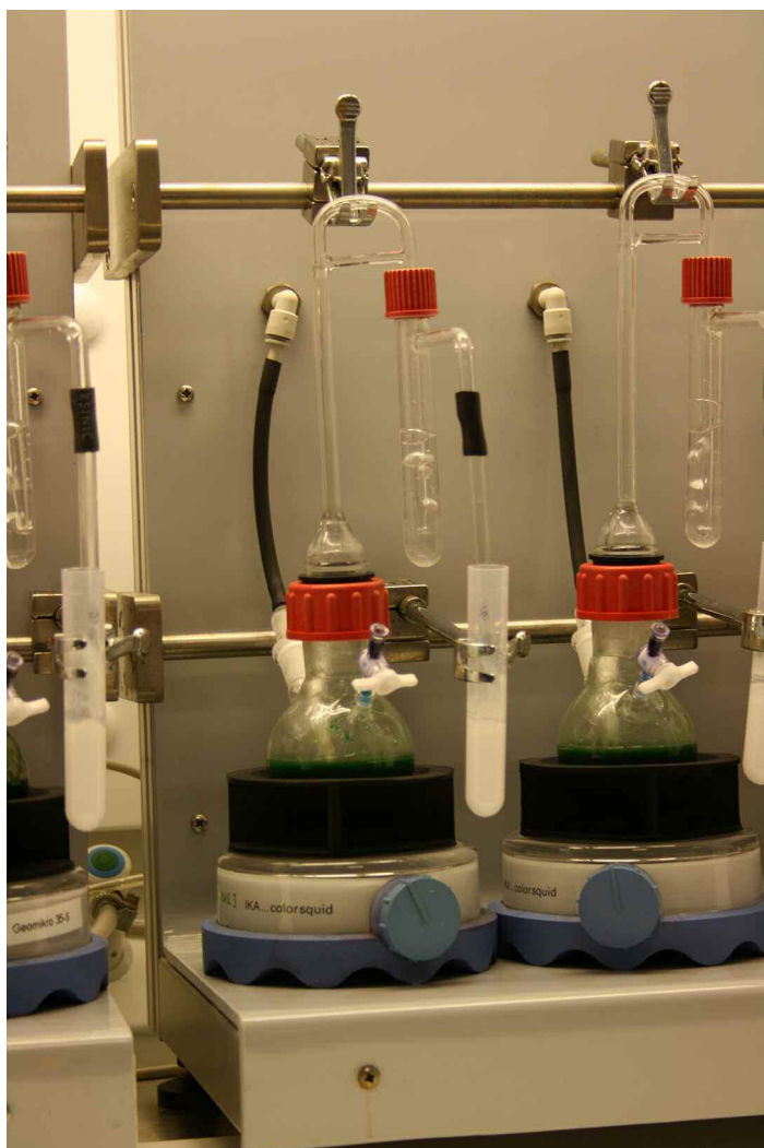
Fig. 2. Distillation apparatus with 1 out of 10 parallel reaction flasks. N_2 enters from the black tube in the back and flushes the H_2S from the reaction flask via the aerosol trap and into the H_2S trap. Here shown with H_2S trapping in a single-use test tube.
