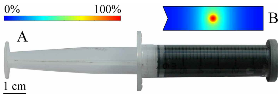
Fig. 7. Example of a sediment sample incubated in a cut-off 5 mL syringe (A). The syringe is closed with a Butyl stopper intended for a crimp-seal vial. B) The modeled distribution of 35 S-TRIS production in the cross section of the syringe after 24 h incubation. 35 SO 4 2- was placed in the center of the core at time zero. The data are normalized to the highest 35 S-TRIS concentration.
